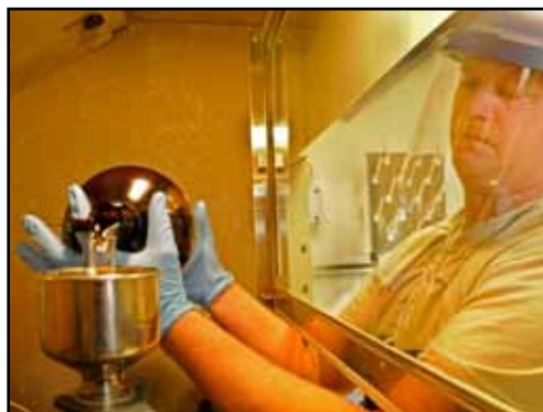
Staff Sgt. James Hubbard pours exactly one gallon of fuel into a filtering device to test for purity. The device uses a vacuum to pull the fuel through a filter.
