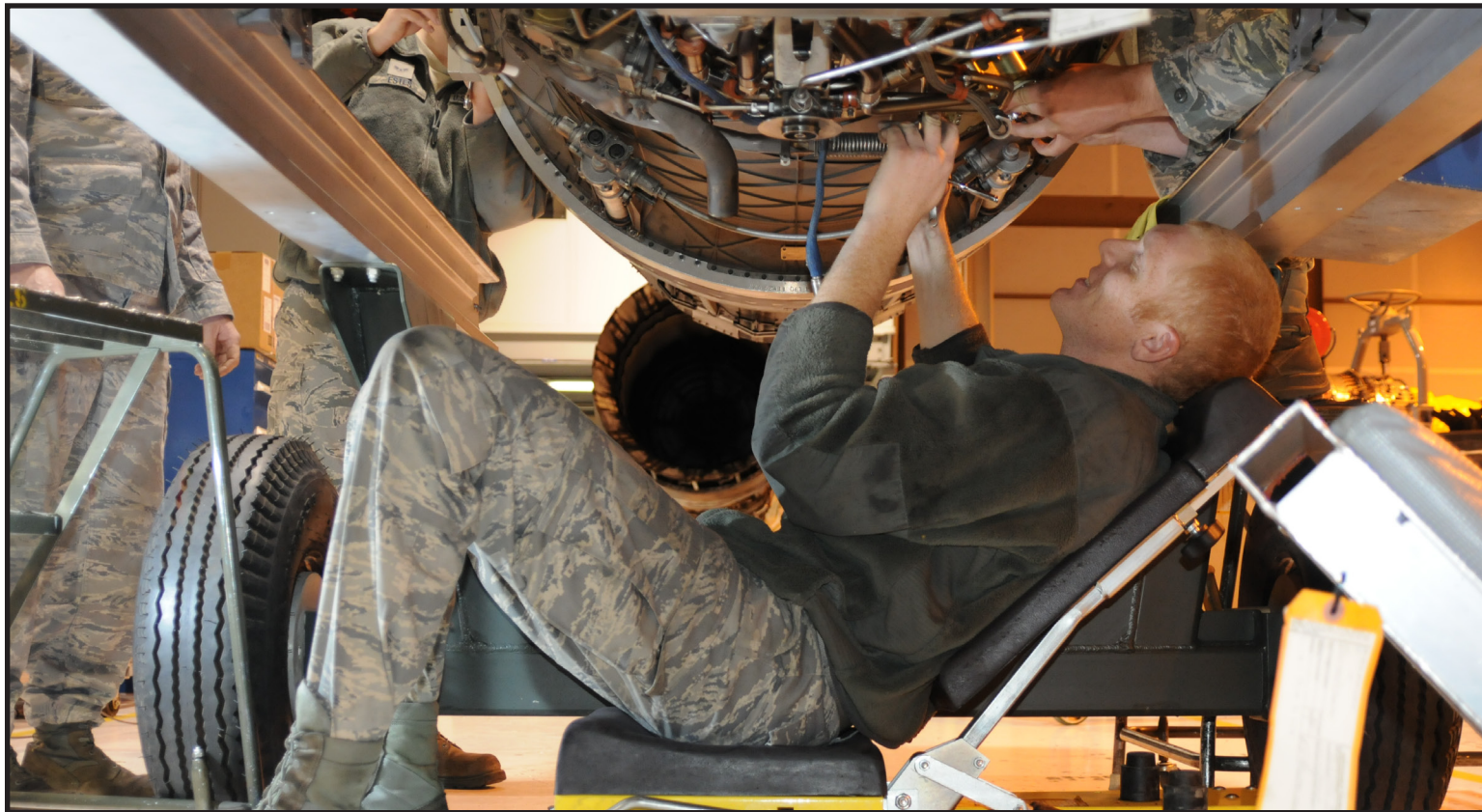
Staff Sgt. Eugene Markgraf works on an F-15C jet engine in a very crowded engine shop Dec. 11, 2012. Maintenance personnel dedicated themselves to refurbishing eight engines packed wall-to-wall in the building due to an unexpected ice foreign object damage incident earlier in the month. (Oregon National Guard photo by Tech. Sgt. Jefferson Thompson)
