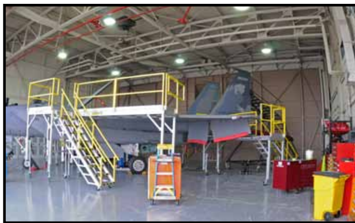
Bld. 400 houses jets in phase maintenance following some renovations to the historic buildings. The stands pictured meet the requirement for passive fall restraint and personnel using them say they speed the phase maintenance process. (U.S. Air National Guard photo by Master Sgt. Jennifer Shirar, 173rd Fighter Wing Public Affairs)
