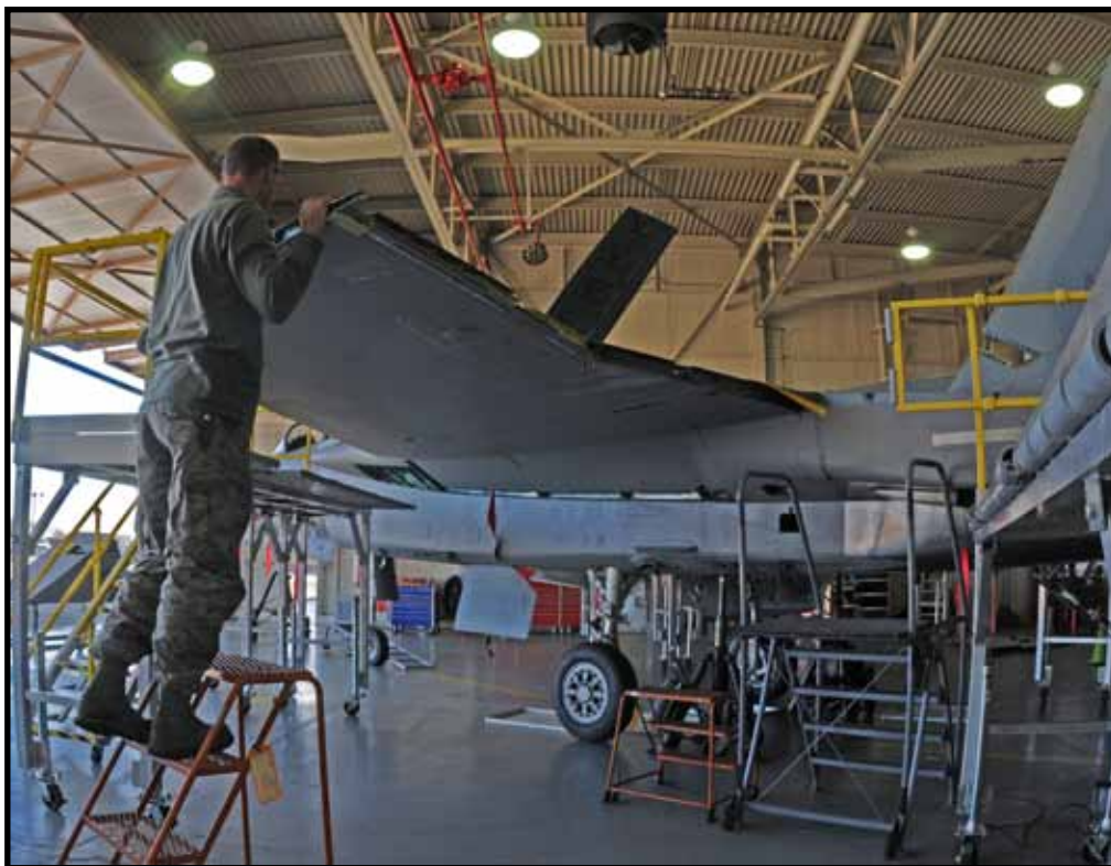
U.S. Air Force Staff Sgt. Andrew Lautenschlager, 173rd Fighter Wing F-15 crew chief, examines the wing of a disassembled F-15 at Kingsley Field, in Klamath Falls, Ore. Oct. 16, 2014. This aircraft is going through phase maintenance where the 173rd FW maintainers closely inspect the aircraft for cracks and other types of damage, verifying that the 30 plus year old aircraft is safe to fly. (U.S. Air National Guard photo by Master Sgt. Jennifer Shirar)
