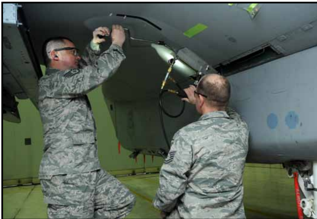
From left, Staff Sgt. James Lovell and Tech. Sgt. Jeff Childs operate a pneumatic drill driving a carbide cutting tool to slowly open a 5-inch by 1/4-inch port in the wing skin where it touches the left wing spar. This opening will allow for routine inspections of that wing spar forestalling a need for depot-level maintenance to remove a large section of titanium plate covering the wing.
