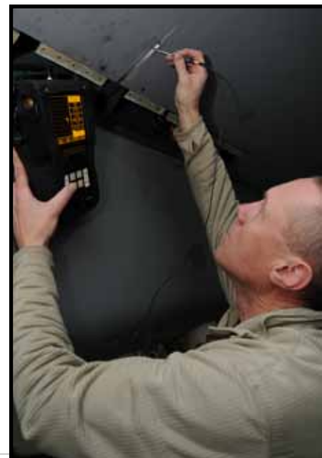
Tech. Sgt. Peter McNally of the non-destructive inspection shop uses an Eddy Current Tester to scan for cracks on the newly exposed section of wing spar.
