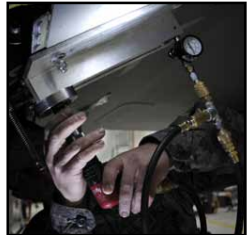
Top: Tech. Sgt. Jeff Childs, 173rd Fighter Wing sheet metals shop, requires a small mirror to help ensure his cutting tool does not cut the wing spar while taking fine cuts measuring only a thousandths-of-an-inch on the skin of an F-15 aircraft wing. While removing the quarter inch of titanium skin covering the wing, the delicate part is ensuring he does not damage the underlying spar.
