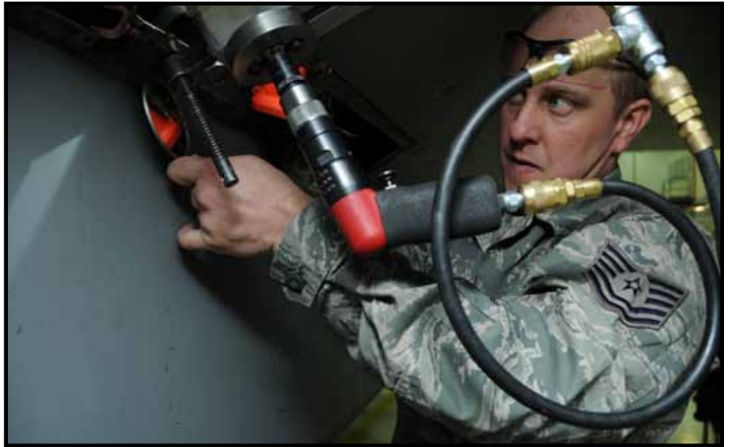
Top: Tech. Sgt. Jeff Childs, 173rd Fighter Wing sheet metals shop, requires a small mirror to help ensure his cutting tool does not cut the wing spar while taking fine cuts measuring only a thousandths-of-an-inch on the skin of an F-15 aircraft wing. While removing the quarter inch of titanium skin covering the wing, the delicate part is ensuring he does not damage the underlying spar.
