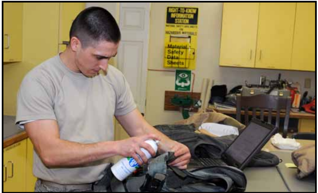
Top: Oregon Air National Guard Staff Sgt. Christopher Hernandez an Aircrew Flight Equipment Specialist assigned to the 173rd Fighter Wing, Kingsley Field, Ore., lubricates fasteners on an F-15 harness responsible for keeping a pilot secure in the event of an ejection.
