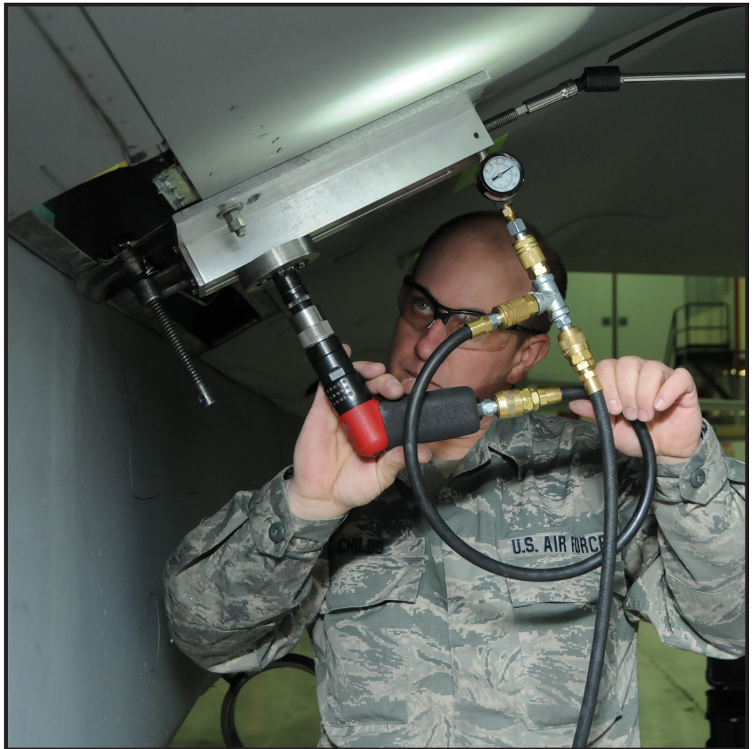
Tech. Sgt. Jeff Childs, 173rd Fighter Wing Sheet Metal shop, removes very thin successive layers of titanium from the skin covering the wing spar on an F-15C aircraft. Time intensive maintenance like this could potentially benefit from a split UTA without the pressure of an active flying schedule. (U.S. Air National Guard photo by Tech. Sgt. Jefferson Thompson)
