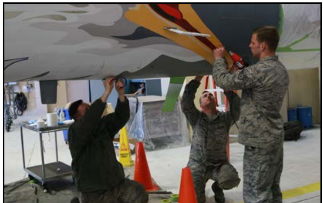
Top: An Airman from the structural shop sands down the black paint after initial tests showed it did not adhere properly to the aircraft. (U.S. Air National Guard photo by Master Sgt. Jennifer Shirar)
