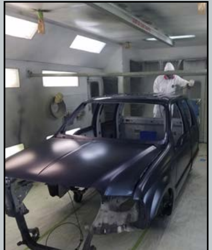
Tech. Sgt. James Childs, 173rd Fighter Wing Vehicle Maintenance, paints the truck cab strata blue. This is part of the new frame of a truck that was totaled in an accident last winter. National Guard Bureau was unable to send a replacement vehicle, so the 173rd vehicle maintenance team decided to completely restore the vehicle to working order from the frame up, a first for Air Force Vehicle Maintenance. (Photo courtesy of 173rd Fighter Wing Vehicle Maintenance)
