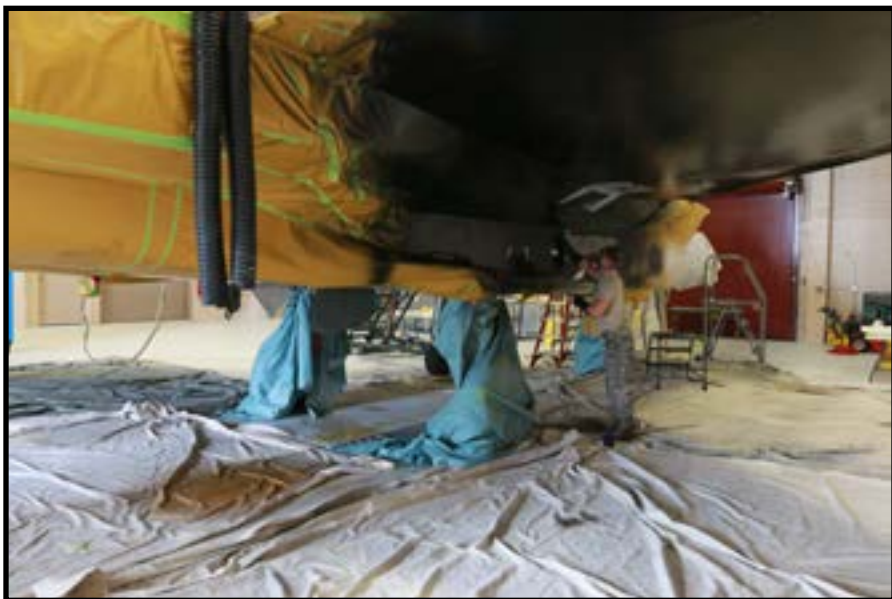
Top: An Airman from the structural shop sands down the black paint after initial tests showed it did not adhere properly to the aircraft. (U.S. Air National Guard photo by Master Sgt. Jennifer Shirar)
